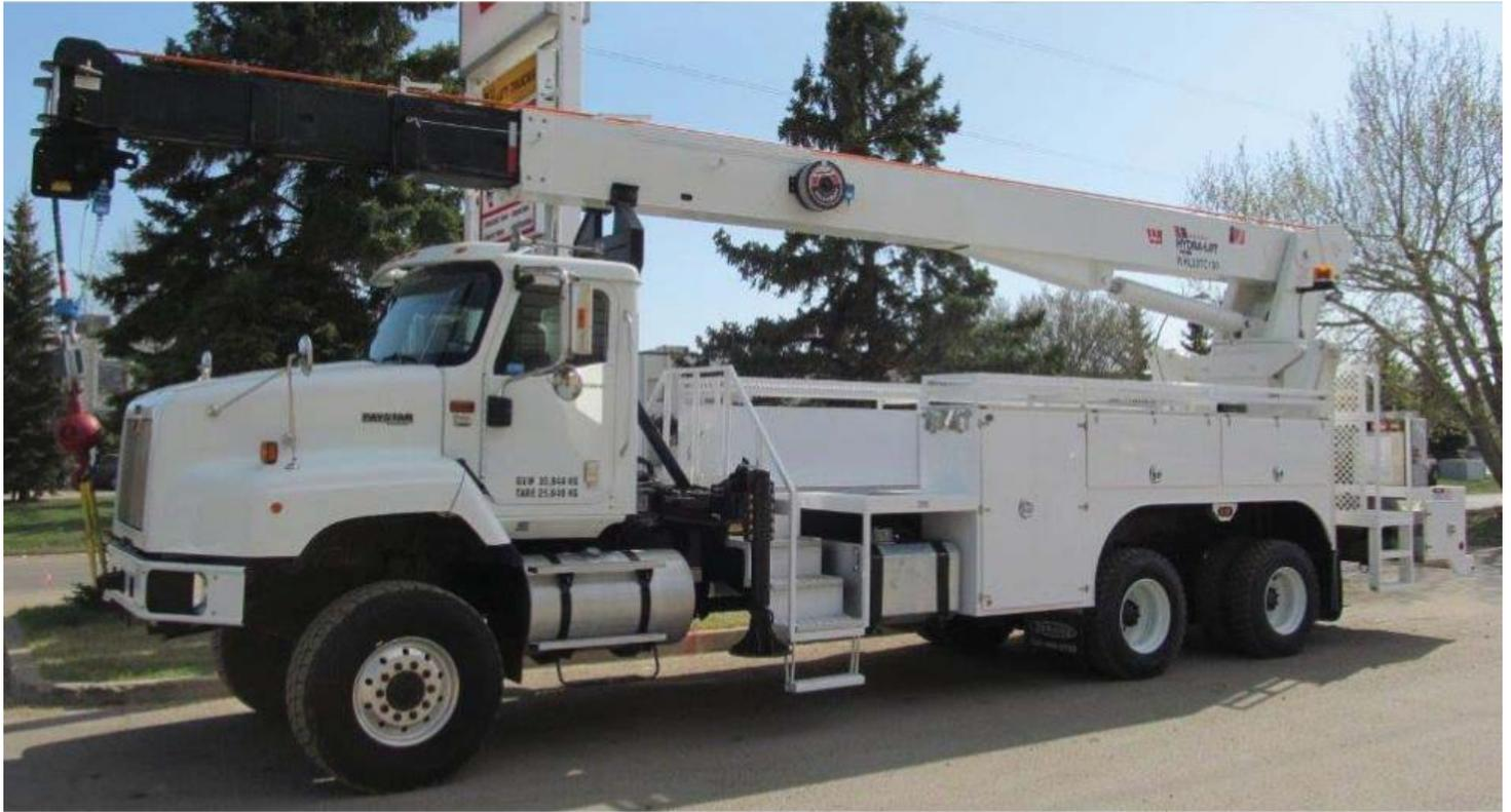
The WHL23TC100 offers a long boom length that provides a distinct advantage on today's modern construction site. The 4-stage dual crowd boom only uses a single cylinder mounted inside the boom.
