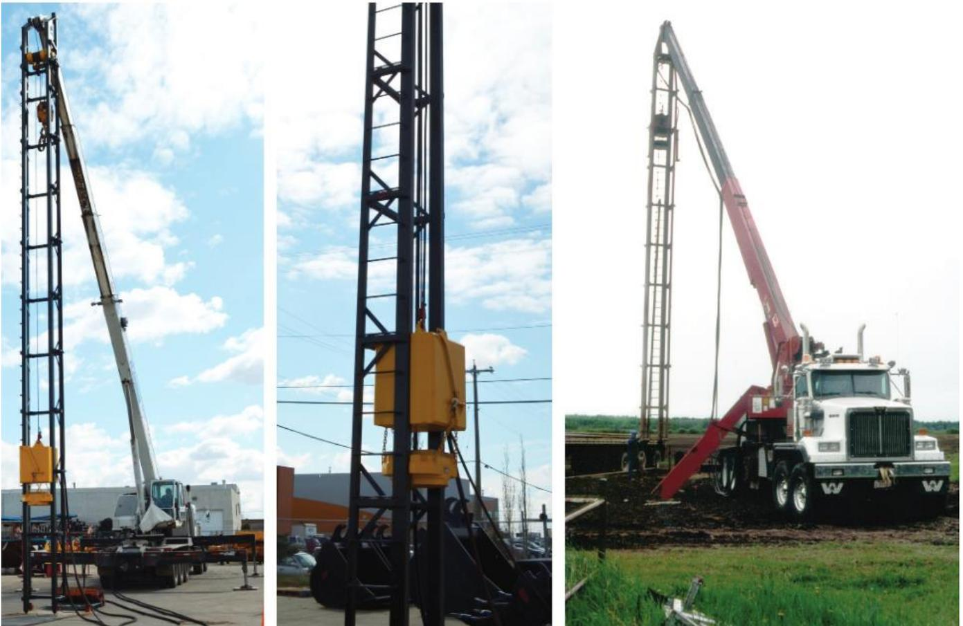
The WHL Pile Driver allows quick and easy conversion from crane operation to pile driving.
