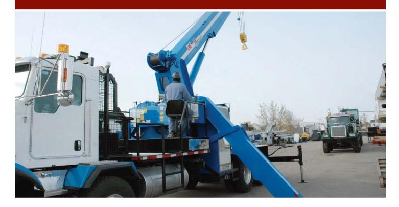
A 30-ton lifting capacity and short stowed boom length makes the HL30TC70 ideal for heavy work in the oilpatch. This crane can be mounted on either a single or double steering axle chassis.
